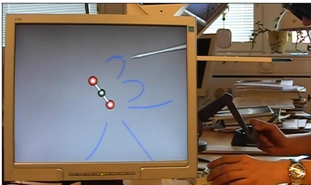
**Figure 3.** Video screenshot from interview conducted with S1 showing five field lines (blue) surrounding a CO<sub>2</sub> molecule. The shot depicts how S1 positions the probe in close proximity to the uppermost field line. The haptic device (right-hand), stereoglasses (top right) and 3-D mouse (left-hand) that the student manipulates during interaction with the model are also shown.
